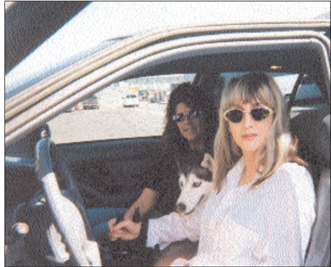
High-tech, adaptive equipment such as this digitally controlled, six-inch steering wheel (under driver's right hand) enables clients to drive independently.
